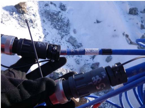
Photo 5: Silver marker marking the corrected identification for the spliced thermistors at station 1+75.
